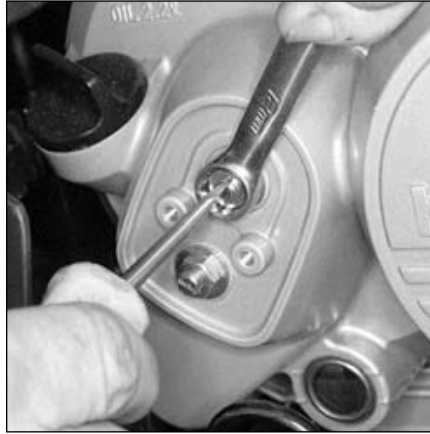
8.3 Loosen the locknut, then hold it with a wrench while you turn the adjusting screw; on 4WD models, adjust the upper screw only
