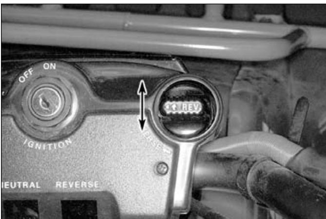
11.2 Rotate the reverse knob and measure freeplay (300 shown; 220 similar)
