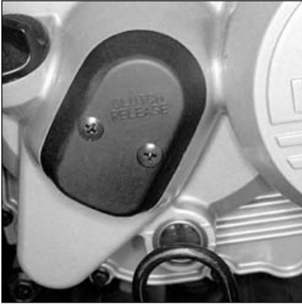
8.2 Remove the screws and take off the clutch release cover (4WD shown; 2WD similar)
