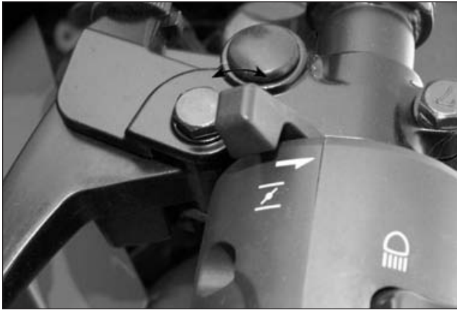
18.14 Check freeplay of the choke lever at the handlebar (EN450 and EX250 models)
