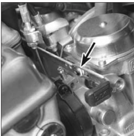
18.16 On EN500 models, make sure the choke plunger lever moves freely and the bushing (arrow) is in good condition
