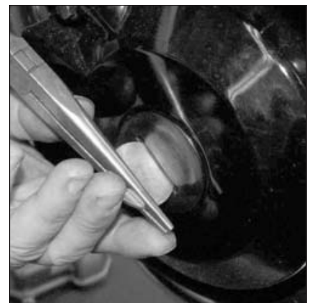
19.5b . . . a coin and pliers will prevent damage to the slots if you don't have a screwdriver wide enough
