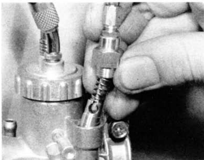
5.1 KH100 models – unscrew choke plunger assembly and disconnect from cable if required
