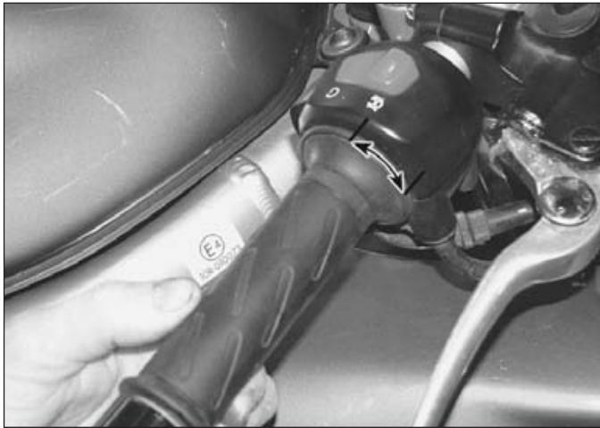
7.3 Throttle cable freeplay is measured in terms of twistgrip rotation
