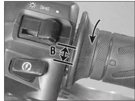
7.3b On GSX-R600W and X models and GSX-R750W and X models, twist the throttle and measure the amount of free rotation (B)
