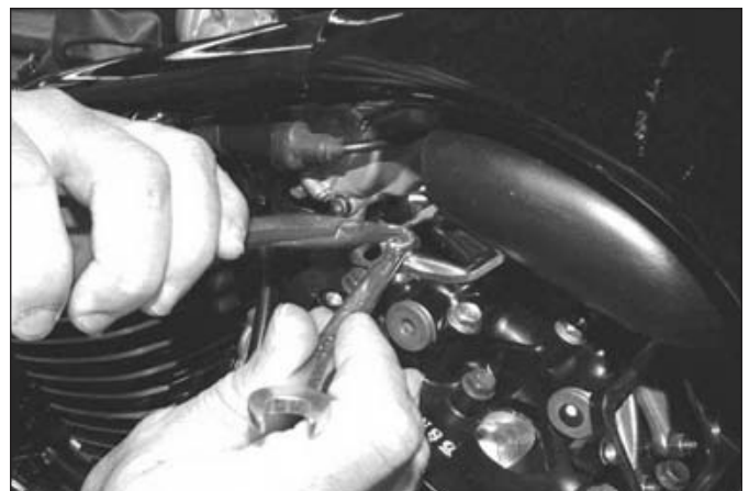
14.16 Hold the lock-nut and turn the adjusting screw
