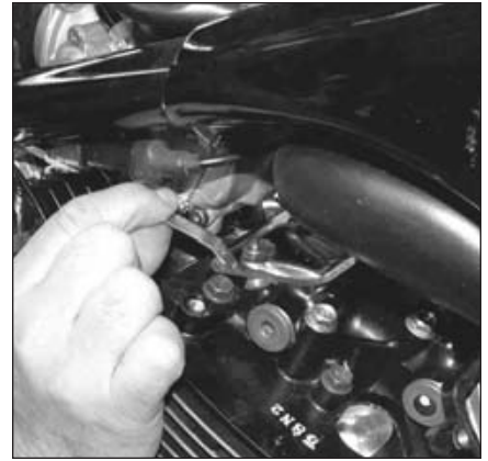
14.13a Slip the feeler gauge between the rocker arm and valve stem . . .
