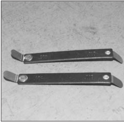
14.12a These offset feeler gauges will make measuring valve clearance much easier . . .
