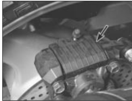
10.9 The brake pads are visible once the dust cover is removed (arrow) - some rear caliper dust covers are accessible from below (rear caliper shown; front caliper similar)
