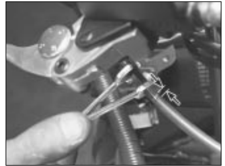
7.8 Loosen the accelerator cable locknut with one wrench, then hold it and turn the adjuster with another wrench to obtain the correct throttle freeplay
