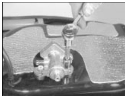
11.8 The fuel tap is secured to the tank by two screws
