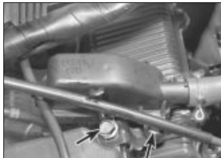
9.3 Remove the mounting screws (arrows) and lift the breather cover off the valve cover
