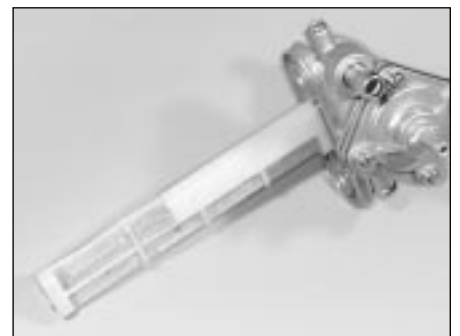
11.9a The fuel filter is mounted on the tap
