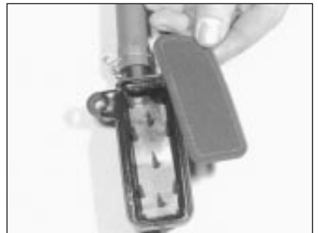
9.4 Remove and clean the foam element
