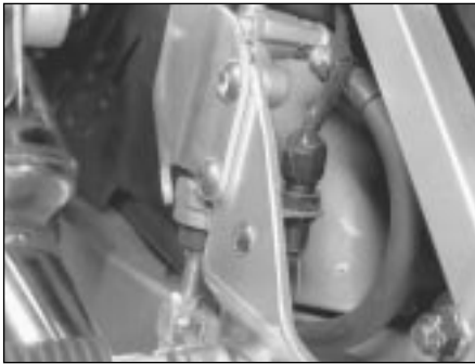
10.7 To adjust the rear brake light switch, raise or lower it in relation to the bracket
