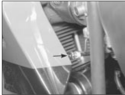
7.3 Turn the idle speed adjusting screw (arrow) in or out until the correct idle speed is obtained
