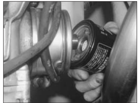
8.7b . . . then install the filter and tighten it as described
