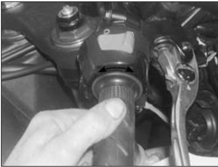
11.3 Throttle cable freeplay is measured in terms of twistgrip rotation
