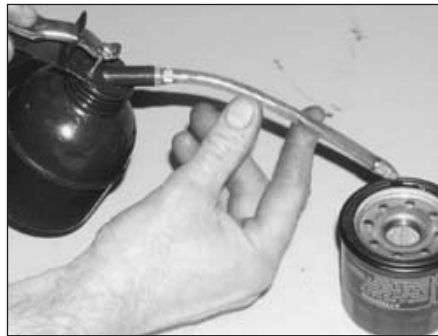
8.7a Smear clean oil onto the seal . . .
