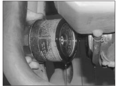
8.6b . . . and allow the oil to drain
