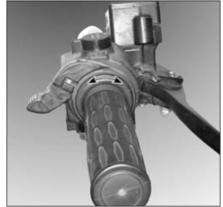
9.2 Check for a small amount of freeplay at the throttle grip (arrows)
