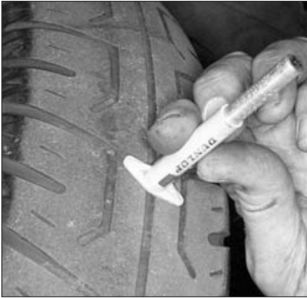
8.2 Measure tread depth; if the raised wear indicators (arrow) are even with the tread surface, the tire needs to be replaced
