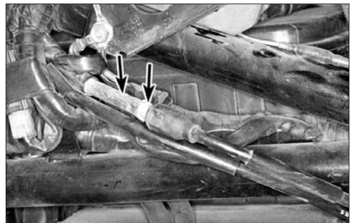
9.4 To make major adjustments, loosen the locknut (right arrow) and turn the adjuster (left arrow)
