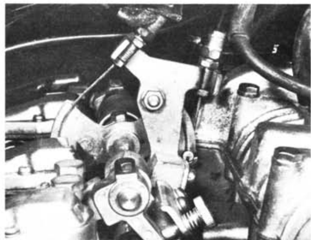
4.2 Pulley operates two cables
