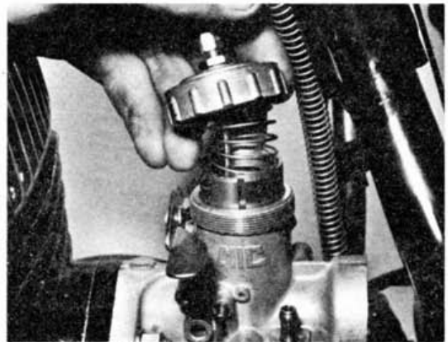
6.13 Carefully slide the throttle valve into the carburettor body (125 shown)
