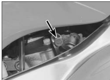
7.4 Idle speed adjuster knob (arrowed) - late models
