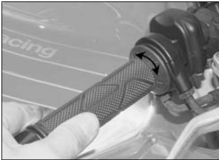
8.3 Twist the throttle and measure the amount of free rotation
