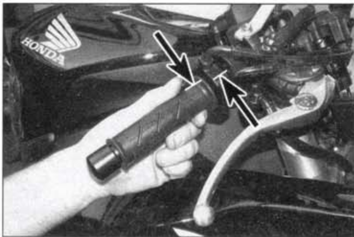
6.4 Throttle cable freeplay is measured in terms of twistgrip rotation
