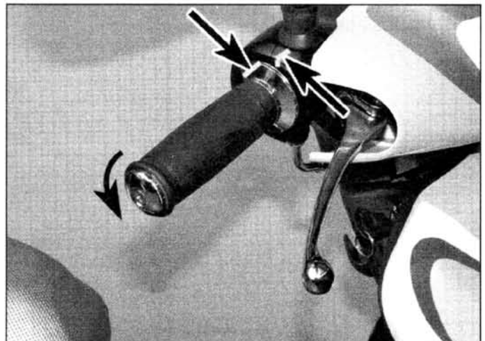
13.3 Throttle cable freeplay is measured in terms of twistgrip rotation
