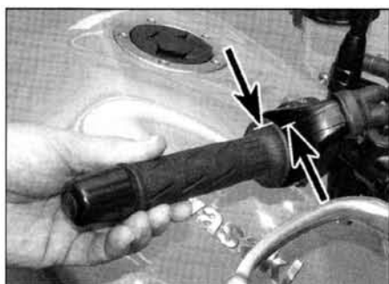
6.4 Throttle cable freeplay is measured in terms of twistgrip rotation
