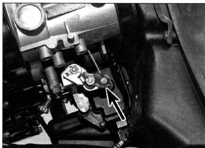
6.7a Check for freeplay at the cam (arrowed) . . .
