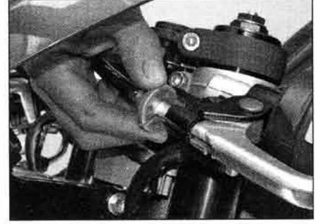
8.5 Adjusting clutch lever freeplay
