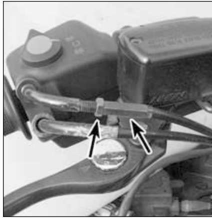
9.3 Make minor throttle cable adjustments at the handlebar adjuster - loosen the locknut (left arrow) and turn the adjuster (right arrow)
