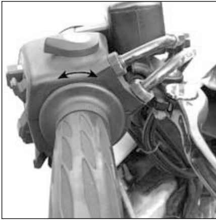
9.2 Check throttle freeplay at the grip
