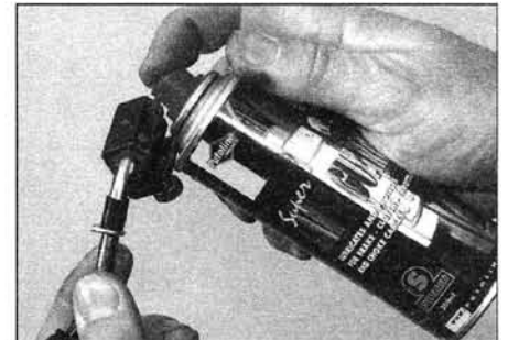
4.15c Connect the can of cable lubricant to the adapter
