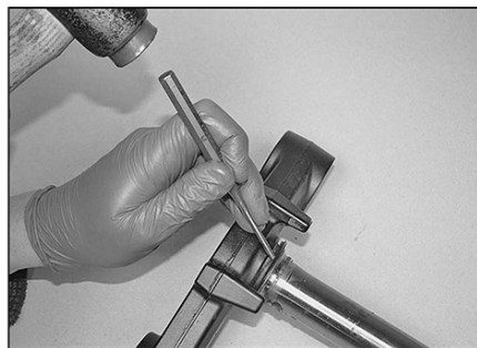
10.6a Dislodge the lower bearing using a cold chisel ...
