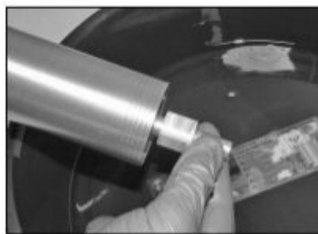
6.40c Pump the damper rod to expel the oil from it
