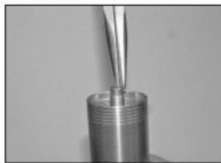
6.41b ... then lift the damper rod out and pump it up and down
