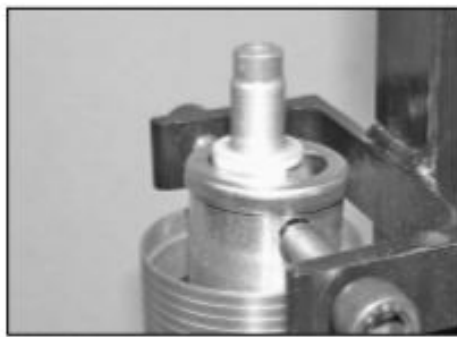
6.45b ... then seat the shaped washer under the rim of the locknut to prevent it dropping
