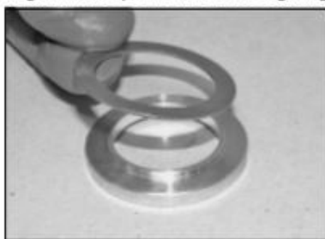
6.42a Seat the washer around the lip and onto the spring seat
