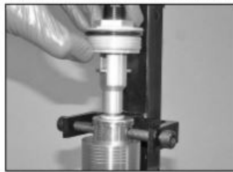
6.46a Thread the top bolt down the rod ...
