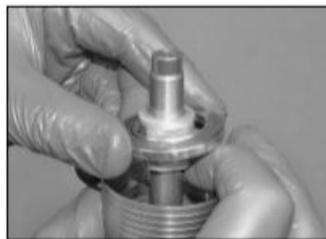
6.42b Fit the seat and/or washer over the rod and into the fork
