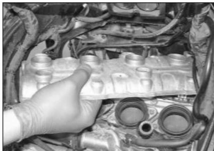
6.6b Removing the valve cover
