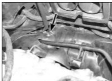
6.4a Undo the screw (arrowed), then release and remove the left-hand section of the duct, noting the routing of the hose
