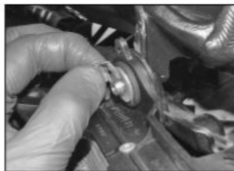
6.4b Release the clip and remove the washer from each side ...
