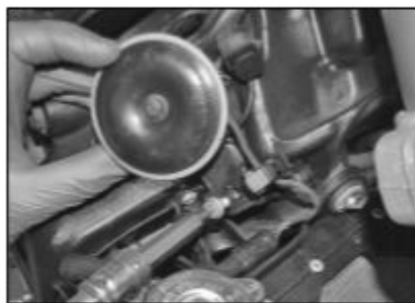
6.5b Displace the horn where fitted on the right
