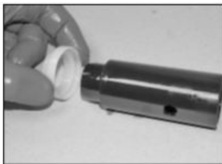
6.43 Fit the seat onto the spacer if removed
