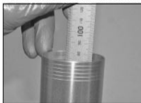
6.41c Measure the oil level
