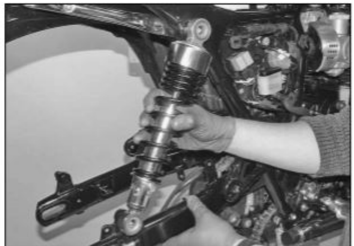
11.3b ... and remove the shock
