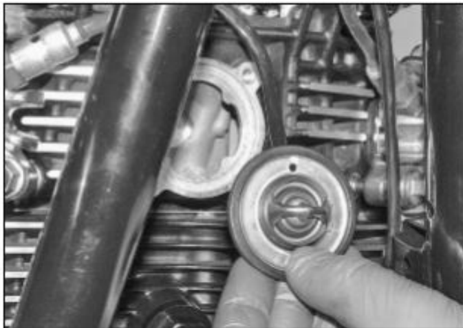
4.3b Remove the thermostat
