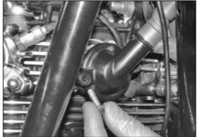
4.3a Unscrew the bolts and displace the cover
