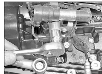
8.15 Unscrew the right-hand tensioner
