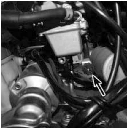
20.3 Adjust the idle speed with the throttle stop screw (carbureted models) or idle air screw (fuel injected models) (carburetor shown)
