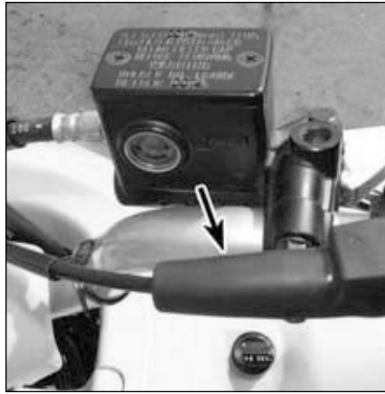
21.4 Slide the rubber boot (arrow) off the adjuster, loosen the locknut and turn the adjuster
