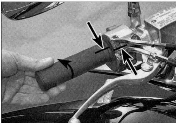
14.2 Throttle cable freeplay is measured in terms of the amount of twistgrip rotation before the throttle opens
