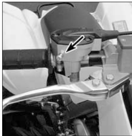
21.7 To adjust the throttle limiter, loosen the locknut and turn the adjusting screw
