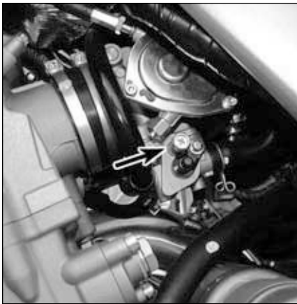
20.3b Throttle stop (idle speed) screw location (700 models)
