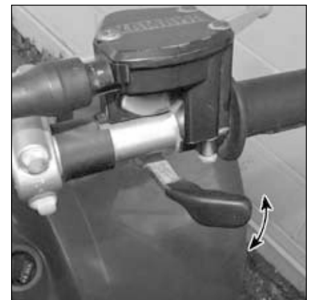
21.3 Check throttle lever freeplay at the lever tip
