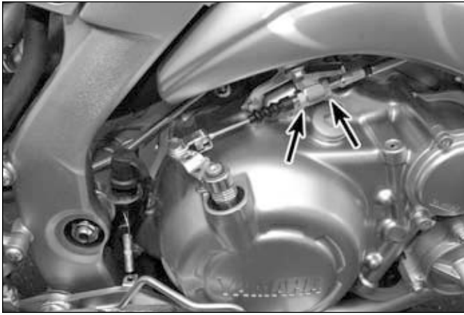
19.4 If freeplay can't be adjusted at the handlebar, loosen the locknut and adjusting nuts, reposition the cable in the bracket to set freeplay, then tighten the nuts
