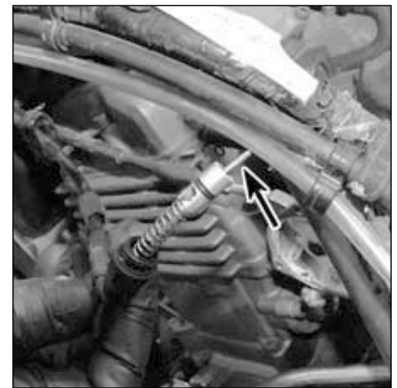
22.3 Unscrew the choke valve from the carburetor, operate the choke lever and measure the stroke of the plunger
