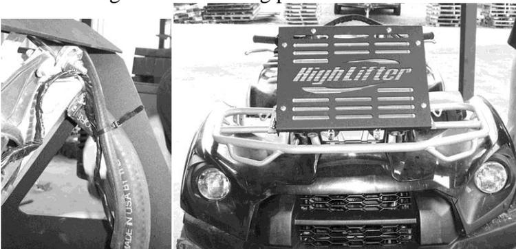
27. Fill the radiator and overflow bottle with factory approved fluid. Make sure that all air is removed from the system.
