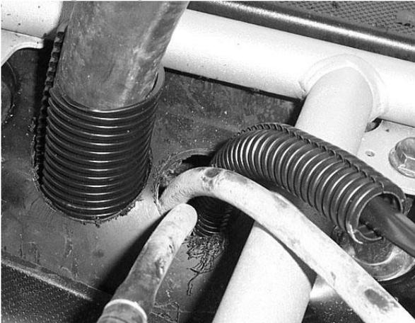
20. Wrap all hoses with the large wire loom and wrap together the overflow bottle lines and wires in the larger wire loom to protect it from cutting and vibration.
