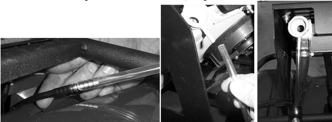
16. Extend the vent from the overflow bottle back up to the filler neck on the radiator and secure the vent line with the zip ties provided. Position the vent line so that it does not vent hot radiator fluid in the direction of the driver.
