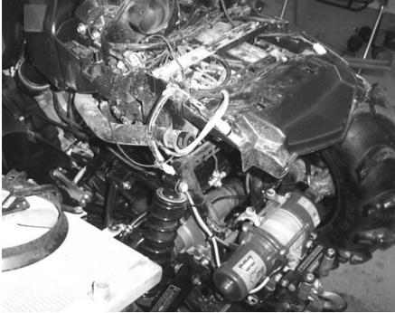
5. Leave stock radiator hoses attached to the engine.
