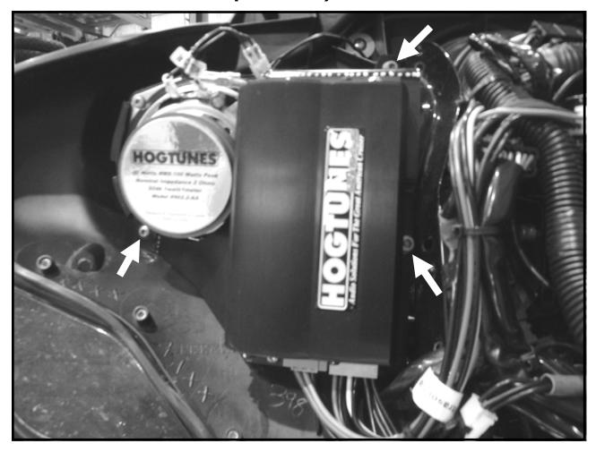
On the brake side of the bike, remove the 3 factory bolts shown by arrows (above), noting the brake side horizontal fairing support bracket will be removed, and not re-installed. Using the supplied fasteners, secure the amplifier to the plate so it is oriented in the same way as the picture above. Put the amplifier/plate assembly in place, and reinstall the 3 factory screws.
