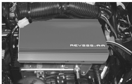
Fig 1.2 Ultra Classic with amp on top of factory CB Module
