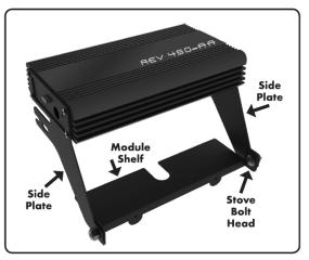
bolts on each side that are farthest away from you (closest to the inner fairing) and remove the bolts closest to you. The amp will "clip in" to the back bolts and the bolts removed will go back in over the plates to secure the amp. Re-tighten all 4 bolts to factory specs. Install the module shelf as shown, noting that the "stove bolt" heads must be positioned as shown. Your module(s) will screw into the shelf using the factory screw(s) you removed from the back of the radio.
