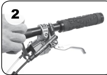
**2** **EN** Disconnect hose at the lever and dispose offluid properly.
