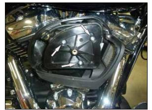
3. Loosen the three air filter retaining bolts as shown.
