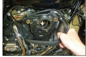
6. Remove the air filter base from the vehicle as shown.
