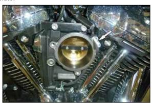
9. Install the long stud as shown ½" down. Note; apply one drop of thread locker onto stud.
