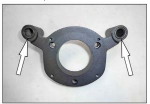
9. Install the remaining two o rings onto the front of the back plate as shown.
