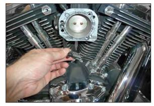
7. Using the provided tie wrap, secure the loose pigtail to the throttle position switch wiring harness. Step 7 is not required on all models.
