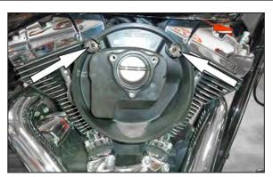
5. Remove the two crankcase bolts as shown.
