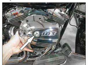
2. Remove the air filter cover retaining bolt and then remove air filter cover as shown. Some models may have a number plate covering the bolts, if so firmly grip edge and remove.
