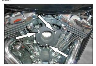
11. Install the provided gasket between the throttle body and back plate use the provided hardware to secure the back plate to the throttle housing. Tighten the crankcase breather bolts.
