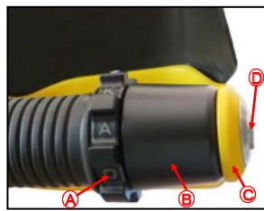
**A**—Friction Nut & Grub Screw
