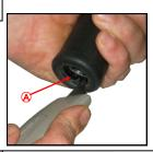
Neatly cut Diameter 25 to 26mm hole in end grip 2
