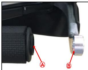
A—OEM bar-end weight removed
