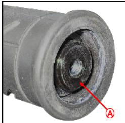
**A**—OEM bar-end weight removed
