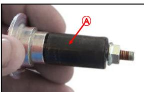
A—OEM Bar-end weight removed
