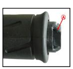
OEM bar-end weight removed with tapered stub
