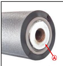
**A**—OEM Bar-end weight removed
