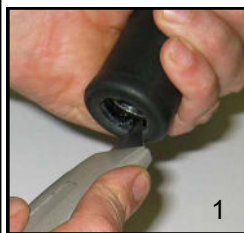
1 Cut approx. 25mm hole into rubber grips
