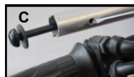
Step C : Fit an M6 bolt into newly exposed threaded insert. Insert is now exposed after trimming throttle sleeve and rubber grip, and then removing the throttle assembly.
