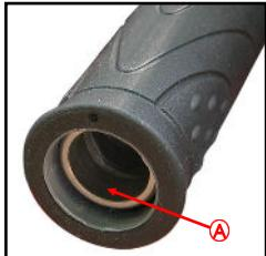
**A**—OEM Bar-end weight removed
