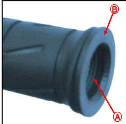
**A**—OEM bar-end weight removed
