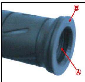
A—OEM bar-end weight removed
