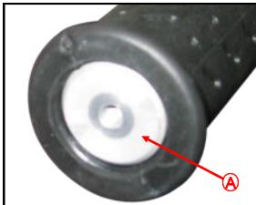
**A**—OEM bar-end weight removed
