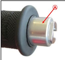
A—OEM End-cap & OEM friction ring removed
