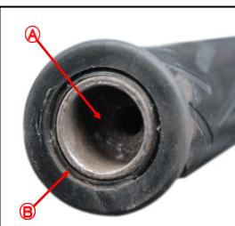
A—OEM bar-end weight removed
