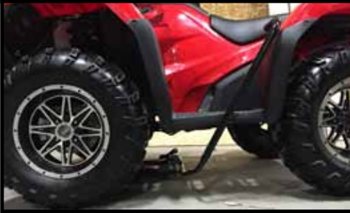
“Figure 12” Manual Lift Install
