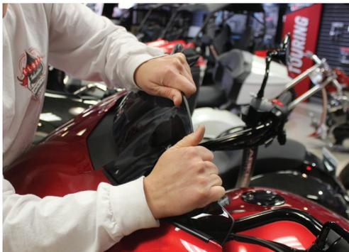
2. Remove the stock windshield and replace it with the new Klock Werks Flare Windshield. Align the holes in the windshield to the mount points on the windshield brackets.
