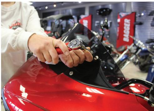
3. Carefully install the hardware removed in step 1 and torque them evenly to 50-60 in-lbs
