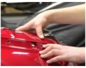
2. Ensure that the inner and outer fairing are aligned so that you can see the brass inserts before installing your Flare™ Windshield.
